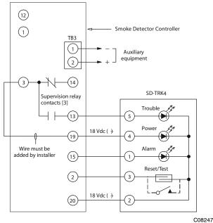
Fig. 24 - Remote Test/Reset Station Connections
